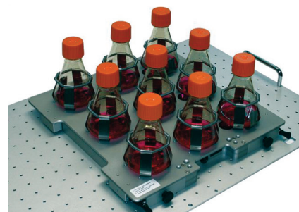
Photo 2: SFR Shake Flask Reader — noninvasive, online monitoring of DO and pH in shake flask culture
