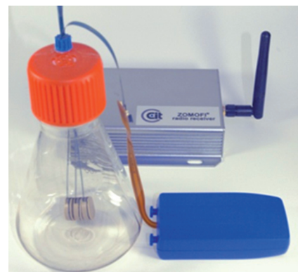
Photo 1: Glucose biosensor integrated in a disposable vessel
