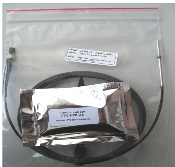
Fig. 2 Flow-through cell pH in a light-tight package, and the respective polymer optical fiber. Both items have to be ordered separately.
