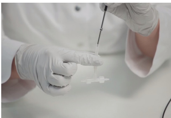
Fig. 6 Mounting the FTC on the polymer optical fiber
