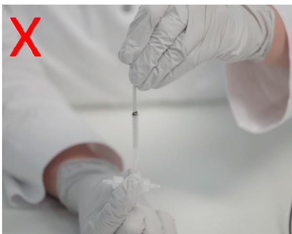
Fig. 7 Wrong handling of the FTC – held at base between connection points
