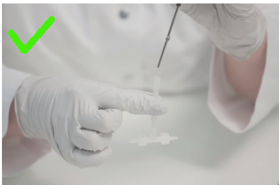
Fig. 8 Correct handling of the FTC – held at the silicon tube for connecting and disconnecting it
