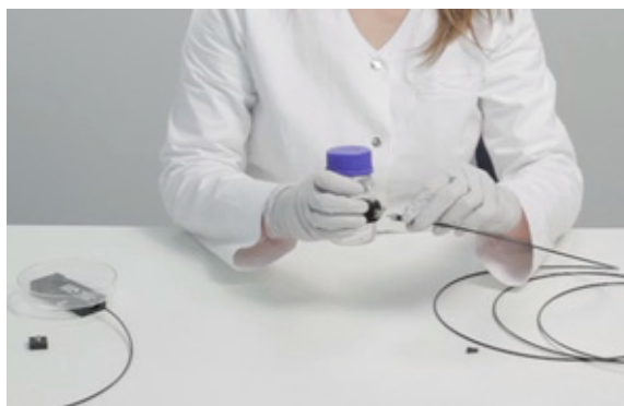
Fig. 12 Connecting the polymer optical fiber to a Adapter for Round Containers ARC
