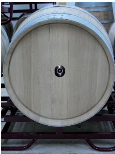
Fig. 3: PSt6 spot placed in a sight glass window in a barrel
