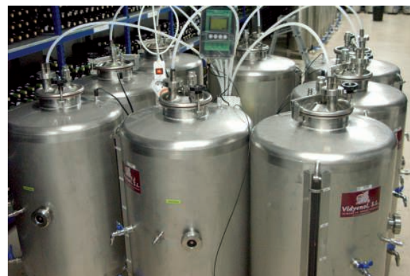
Fig. 2 Monitoring red wine in tanks during the MOX process.
