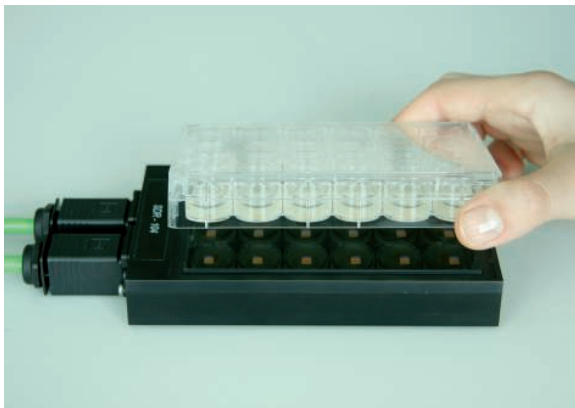
Fig. 1 The new SensorDish® Reader for non-invasive on-line monitoring of oxygen in cell cultures.
