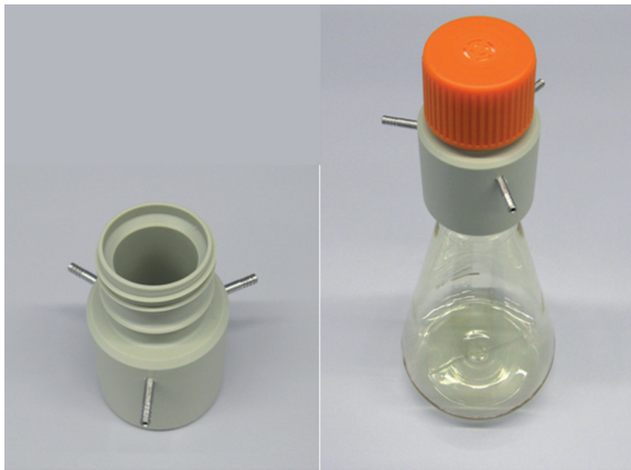
Fig. 2: Adapter prototype w/o (left) and w/ shake flask (right).
