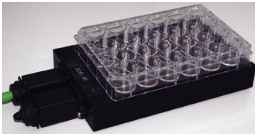
Photo 1: Sterile online monitoring of pH and oxygen in CHO-S cultures is made possible by the new SensorDish Reader instrument from PreSens. Optical sensors are located at the bottom of each well of a 24-well multidish and read by a small and robust 24-channel reader.
