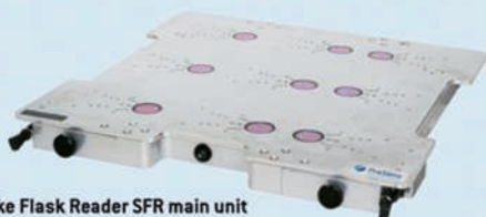
Shake Flask Reader SFR main unit
