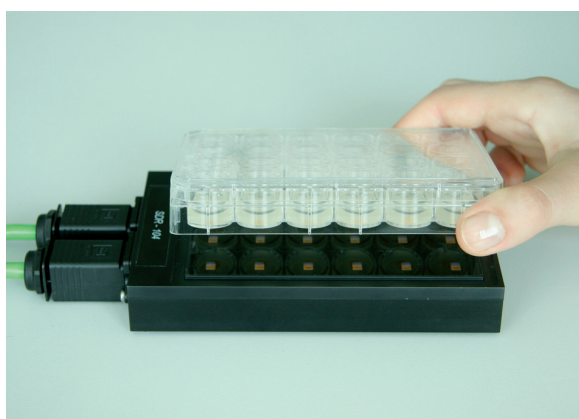
Fig.1 Non-invasive online monitoring of oxygen in bacterial culture samples using the new SDR SensorDish® Reader.
