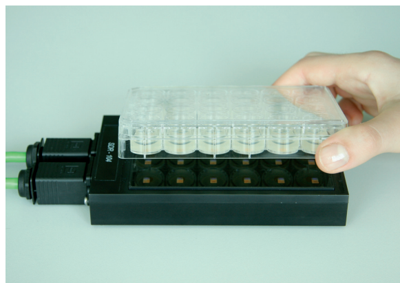
Fig. 1 SDR SensorDish® Reader for online monitoring of dissolved oxygen and pH in 24-well multidishes.
