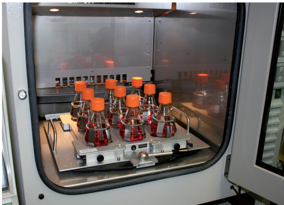
Fig. 1 SFR Shake Flask Reader on shaking platform in incubator. Integrated dual optical sensors enable non-invasive simultaneous measurement of dissolved oxygen and pH.
