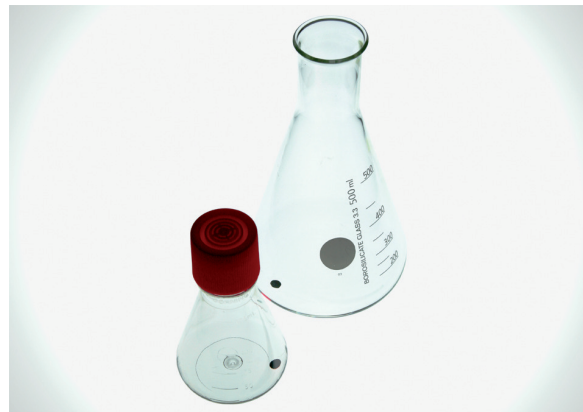
Fig. 2 The directly useable SFS plastic flask contains disposable pH and oxygen sensors. Glass flasks only contain autoclavable oxygen sensors.
