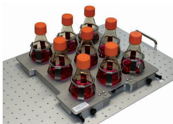
Fig. 1: SFR Shake Flask Reader
