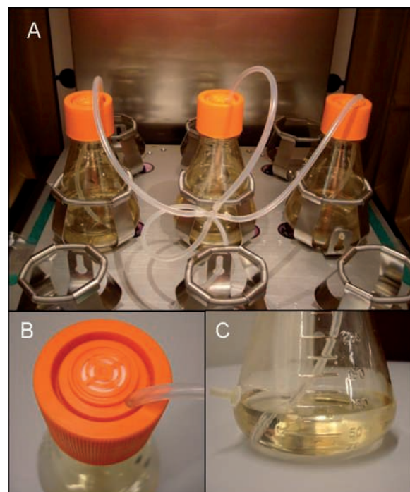
Fig. 1 Experimental set-up for the determination of k_L a values. (A) gassing-out with N_2 by a silicone tube inserted through a hole in the vented cap (B). After purging with N_2 the silicone tube (C) was withdrawn in order to replace the headspace with air.
