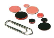
Sensor spots are the most versatile version of non-invasive optical oxygen sensors. They can be attached to the inner surface of any transparent glass or plastic vessel like e. g. used for packaging. Oxygen is measured contactless through the transparent vessel wall. The SP-PSt6-NAU has a measurement range of 0  $-5\,\%$  oxygen, dissolved or in the gas phase. The oxygen sensitive coating is immobilized on a 125  $\mu m$  flexible transparent polyester foil, which does not stand autoclaving.
