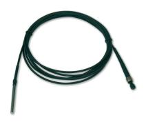
The  ${\rm CO_2}$  dipping probe DP-CD1 is an optical sensor based on a 2 mm polymer optical fiber. The end of the probe is covered in a high-grade steel tube. It is the solution for invasive measurements and monitoring of dissolved  ${\rm CO_2}$ .
