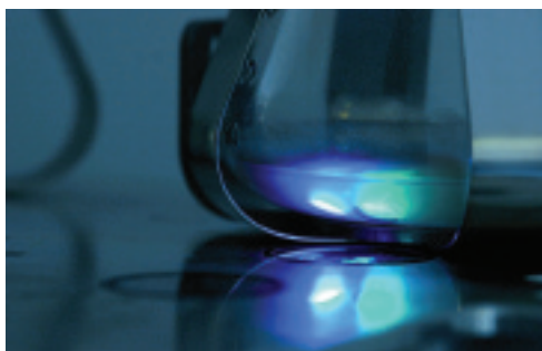
Figure 1: Chemical optical sensors integrated in a shake flask; the fluorescent dyes are excited with light of a certain wavelength and the sensor response is read out by the shake flask reader
