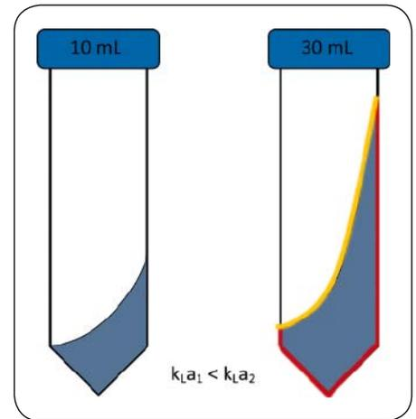
Fig. 3: Schematic illustration of fluid behavior at higher shaking frequency, 50 mm amplitude, and different filling volumes (left: 10 ml, right 30 ml); the specific exchange area (yellow line) and the contact area (red) increase with larger filling volume, which enhances oxygen transfer.
