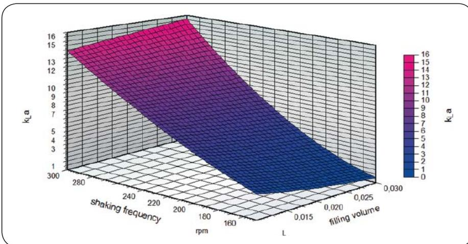
Fig. 2:  $k_La$  values at a set amplitude of 50 mm with varying filling volumes and frequencies. With increasing frequency the  $k_La$  value is no longer influenced by the filling volume; this model does not show that  $k_La$  values increase with larger filling volume and higher rotation speed.
