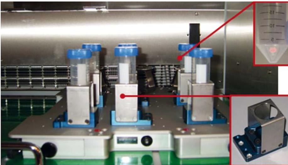
Fig. 1: Bioreactors on the SFR; upper inset: integrated sensor spot for DO measurement; lower inset: holder designed for tube bioreactors
