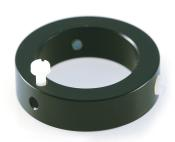
The Vial Adapter is used to attach the POF (polymer optical fiber) to a 20 mL SensorVial (special glass vial with integrated oxygen sensor foil) using a screw. It can be attached to the vial in different heights for measurement in the liquid phase and the headspace and can also be used in a water bath. The POF is available as a separate accessory.
