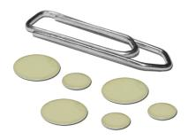
The CO<sub>2</sub> sensor spots measure the partial pressure of dissolved carbon dioxide. The spots are fixed on the inner surface of glass or transparent plastic vessels. Measurements are then taken contactless from the outside through the transparent container material.
